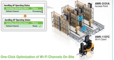
On-site environments can be drastically different from test environments. Operators need to adjust the Wi-Fi channels of devices for each on-site scenario to find the best channel for wireless communication. Moxa's AeroMag technology features a channel optimization function, which searches for and sets up the best Wi-Fi channel for your devices based on your on-site environment.
